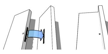
LAMELLO Unlike traditional cam fixings, the fixings we use are designed not to be seen when the unit is assembled. To fit them, simply align the pair of fixings, and use an allen key in the adjacent hole to join twist the lever from one into the other.
