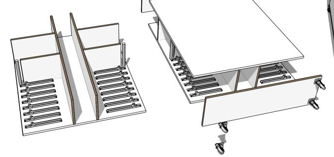
Unlike traditional cam fixings, the fixings we use are designed not to be seen when the unit is assembled. To fit them, simply align the pair of fixings, and use an allen key in the adjacent hole to join twist the lever from one into the other.
