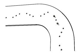
There are two different types of holes on the 'boomerang' panels – blind holes (that do not go all the way through) and through holes (that do).
