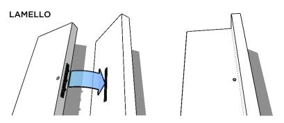
Unlike traditional cam fixings, the fixings we use are designed not to be seen when the unit is assembled. To fit them, simply align the pair of fixings, and use an allen key in the adjacent hole to join twist the lever from one into the other.
